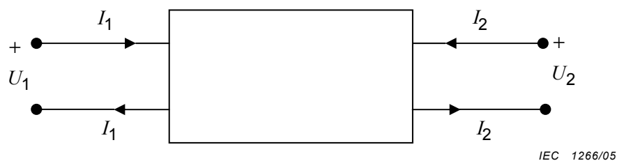
Figure 1 – Conventions concerning signs in electric circuits
